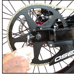
Chain tensioner nut 13mm
