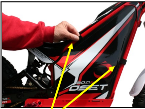
(1.) Release Velcro straps
